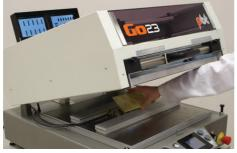
Pneumatic clamping of print frame with thickness up to 40 mm.
