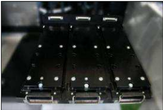
CLM Feeder rack with Feeder Base Plate
