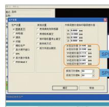
Form a closed loop system with SPI on line, when after receiving the SPI printing bad feedback, the machine will automatically adjust automatically according to the offset of SPI feedback, x, y direction deviation can automatically adjust to complete within 3 PCS, and clean Stencil, improve printing quality and production efficiency, form a complete printing feedback system.
