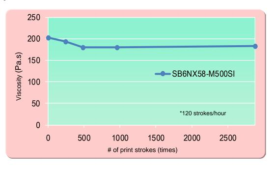
Viscosity shows little change after continuous kneading thanks to the optimal combination of activator constituents.
