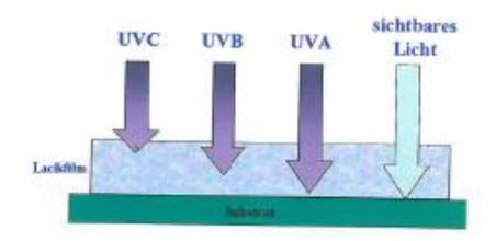
Curing depth within the coating layer is depending on the UVA, UVB and UVC.
